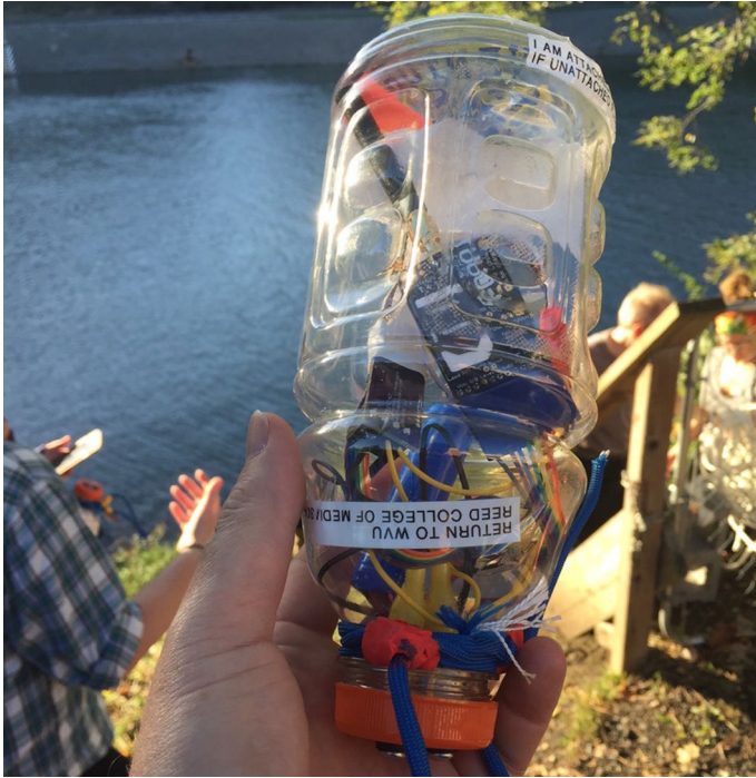
Fig. 8 RIFFLE conductivity and temperature prototype used in John Keefe's West Virginia deployment
