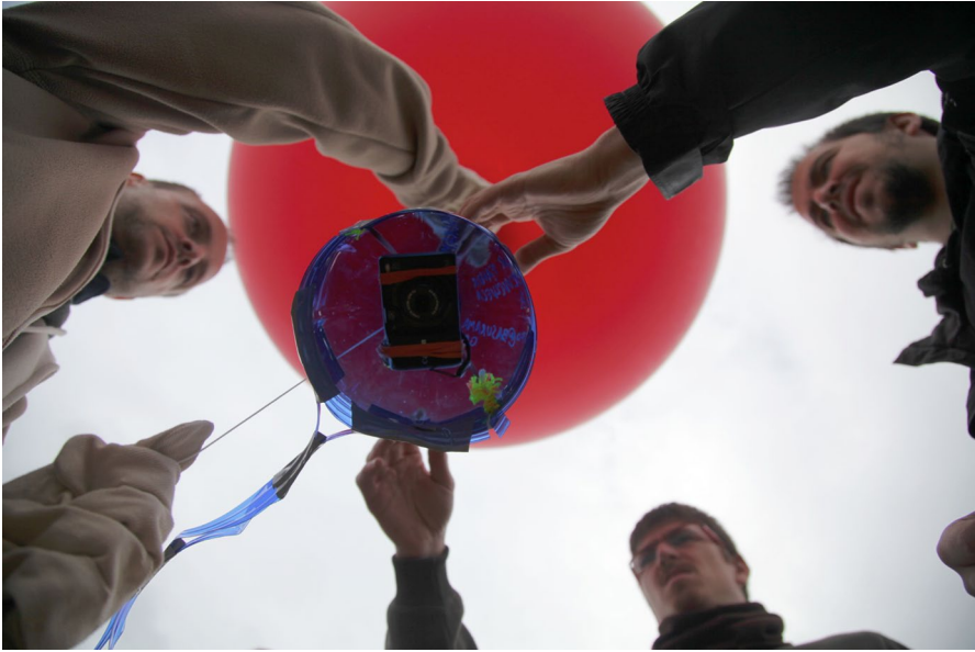
Fig. 2 Setting up the camera in a plastic bottle rig developed by Public Lab and attaching it to the balloon. The camera is set on “continuous mode” and takes pictures in short intervals during the time it is in the air
