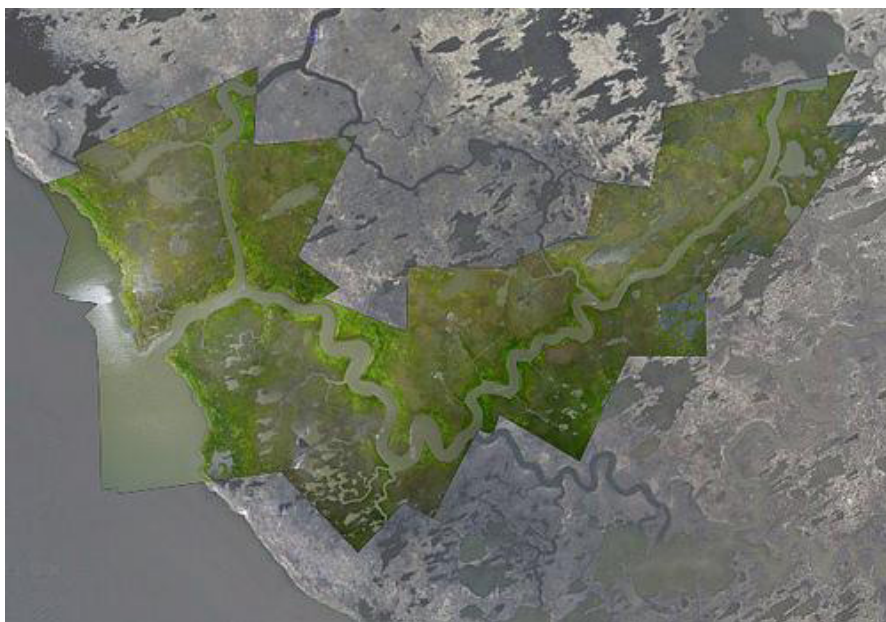
Fig. 2A - A Public Lab map of Lake Borgne, Louisiana, made using open source photo stitching and rectification software MapKnitter.org and Public Lab's balloon mapping 7 techniques. Photos (green, colored strip) were taken via balloon by Erin Sharkey, and stitched together in MapKnitter (using underlying Google Maps satellite imagery as a base layer, for rectification) by Stewart Long.
